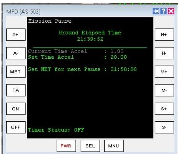
The Time Acceleration value can be also be changed with the A+ and A- buttons. Setting the Time Acceleration will not change the Current Time Acceleration until the timer is turned on.
