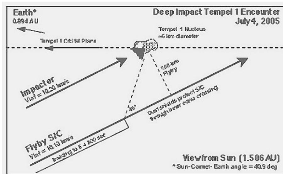
During the encounter, the Flyby Bus continues imaging until approx. 700 km altitude, at which time the spacecraft is reoriented so that the dust shielding provides protection during the crossing of the inner-coma.
