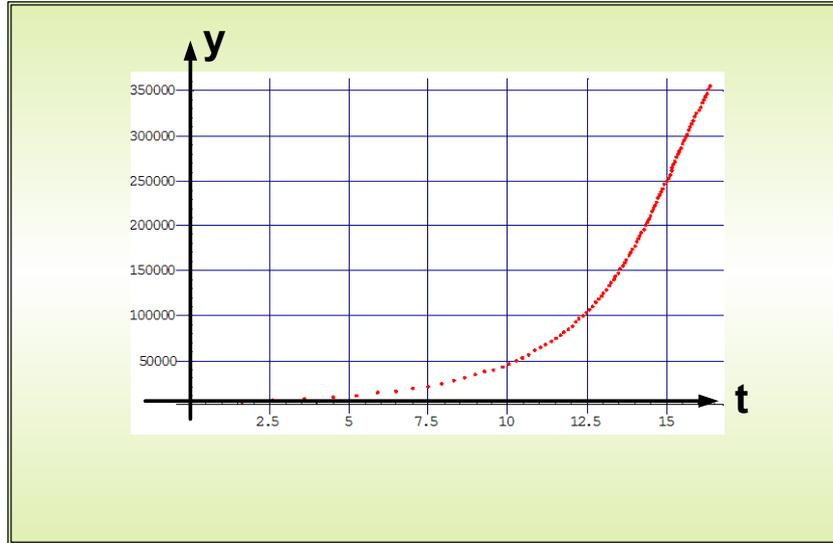
Fig. 4 : The variation of the y coordinate with time along gravity turn path with:
