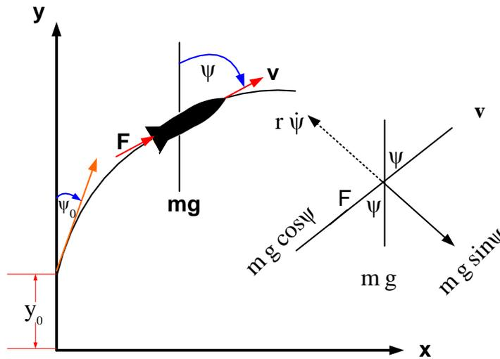
Fig. 2 : Gravity turn trajectory
