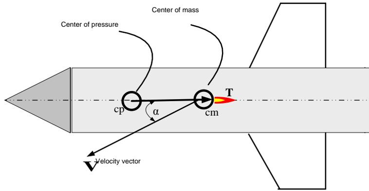
Fig1 : The angle of attack
