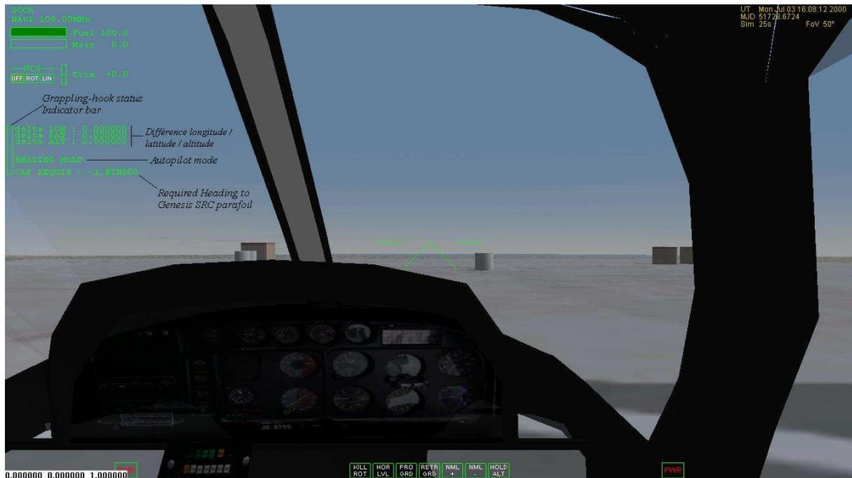
**Green Side-bar:** Raised / Lowered position of the grappling-hook.
