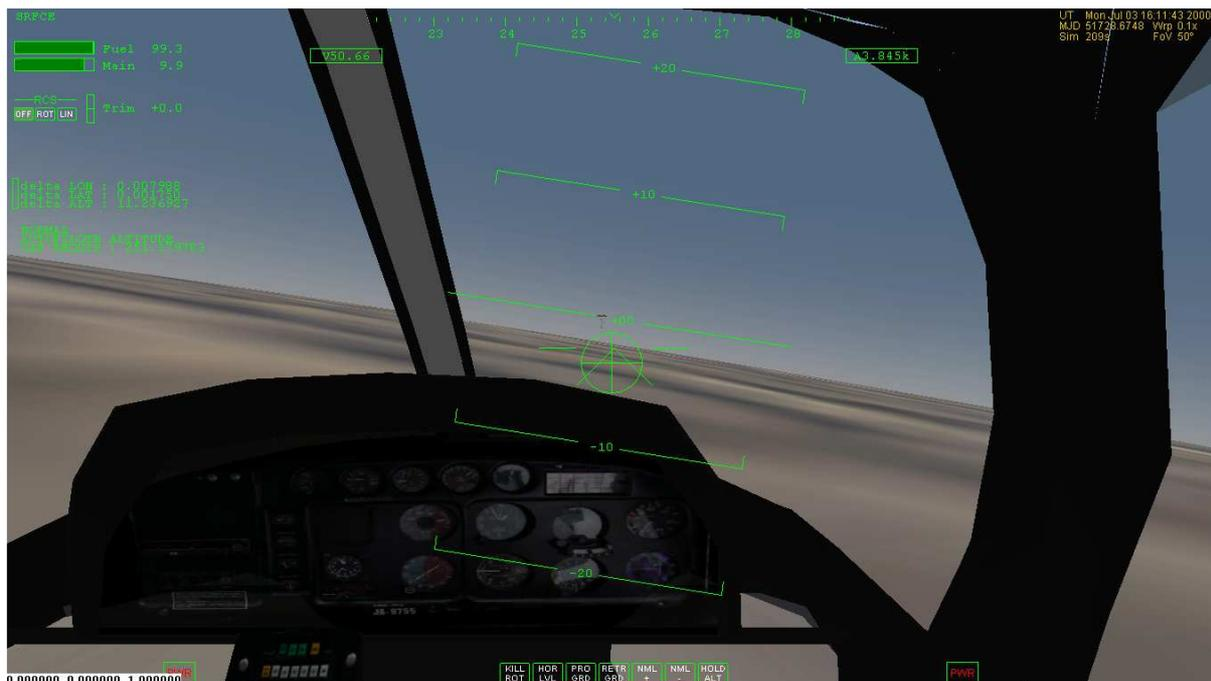
Here you can see the green side-bar indicates the grapple-hook is lowered and the delta long/lat/alt display shows the angular difference of longitude  $0.007988^\circ$  and latitude  $0.001750^\circ$  between the as350 and Genesis SRC parafoil. The difference of altitude is 11.23 m, showing that we are above the capsule. (Ideally, you should be between 15 and 20 m above the capsule to snag the parafoil with the grapple-hook. Otherwise, you will have to go around again).
