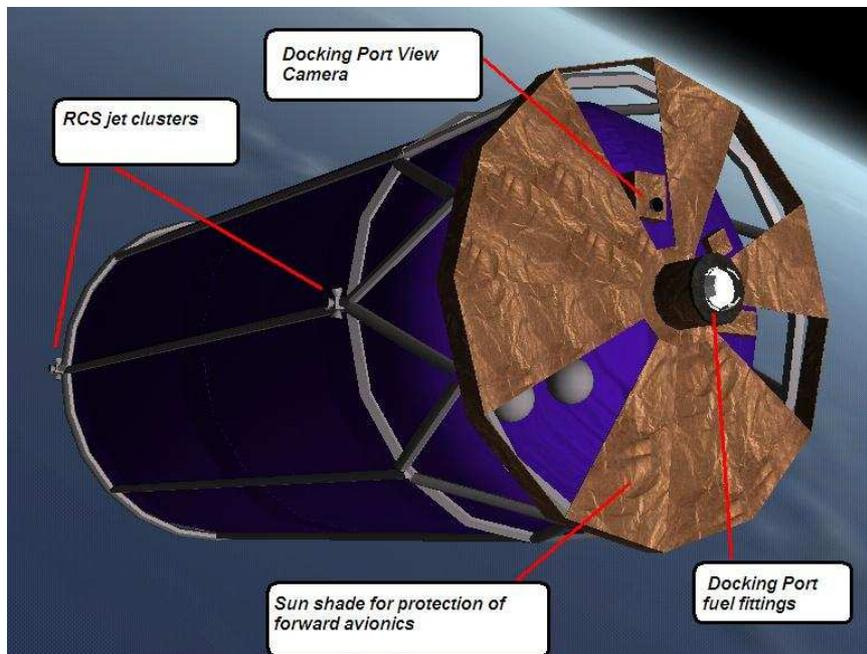
The pilot (you) flies it remotely using the camera installed on one of the avionics boxes protruding through the gold foil sunshade on the bow. This means that when docking, your point of view will not be on the centerline, but rather just above and to starboard of the docking port. If you tilt your view down and to the
