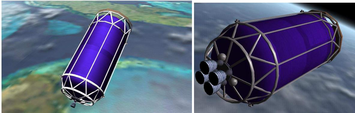
The Jumbo Tanker is an unmanned spacecraft designed to carry propellant into Low Earth Orbit (LEO) and deliver it to a rendezvous target, be it a station, a ship, or just a particular parking orbit.
