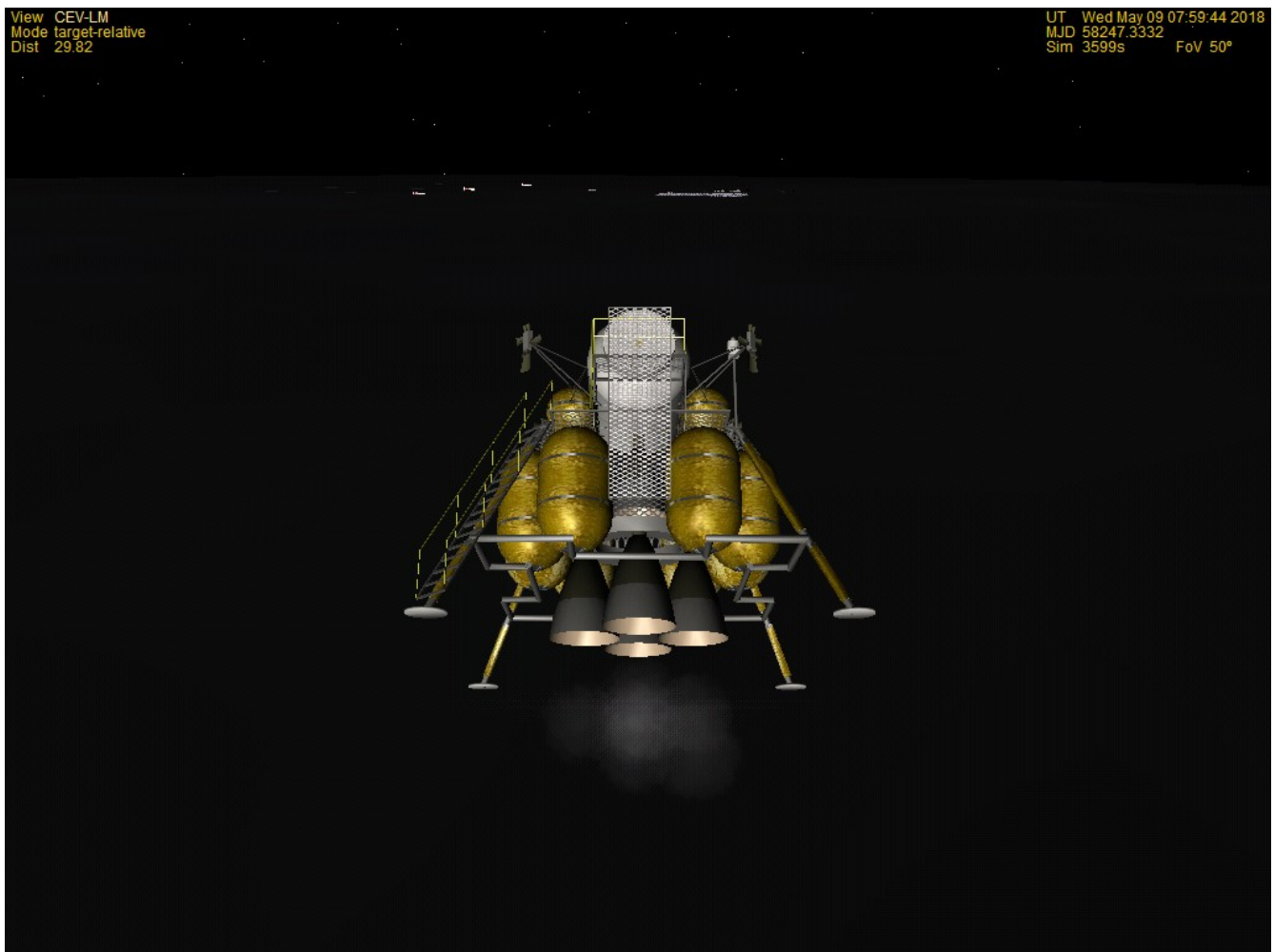
Figure 5: Hovering towards a base. The LM is pitched down to cause a forward acceleration.
