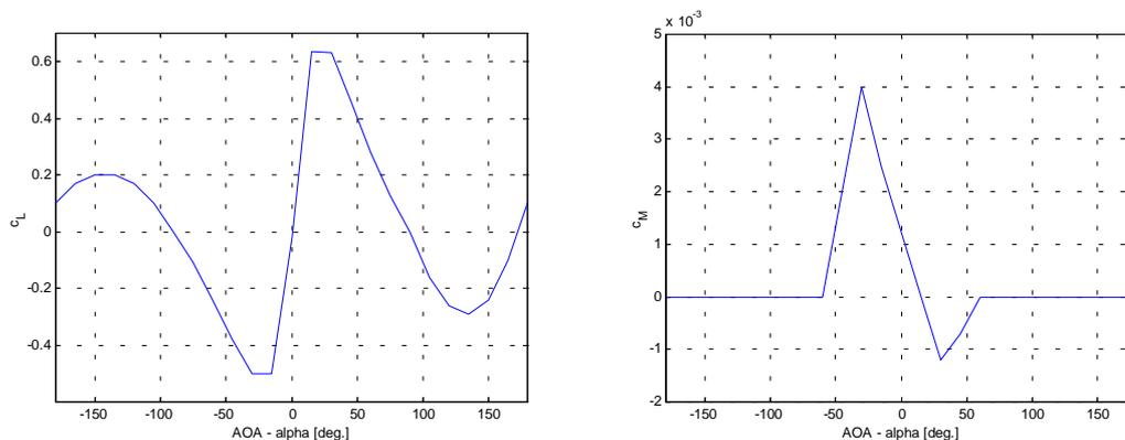
The lift profile utilises a documented lift slope of 0.0437/deg. Everything else is rather ad-hoc. In particular the moment coefficient profile needs more thought. Other parameters:
