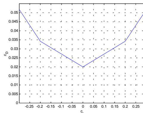
The horizontal lift profile is symmetric (symmetric airfoil). Other parameters:
