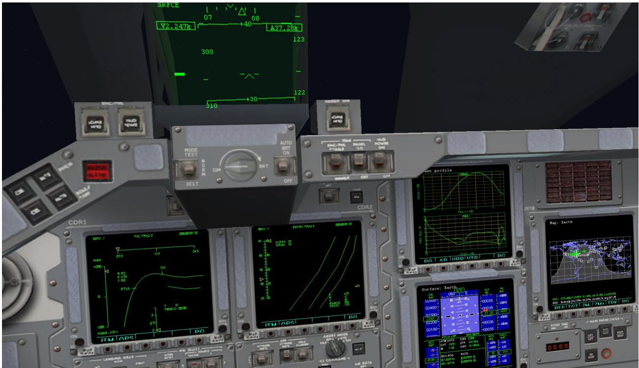
Fig.15 - Nz Hold phase. Check the Acc value on the SRF MFD within limits (target is 25m/s²) Alpha is lowered accordingly
