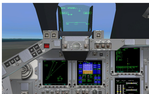
Fig.22 - Up/down and left /right the final to touchdown sequence - Note the HUD info displayed
