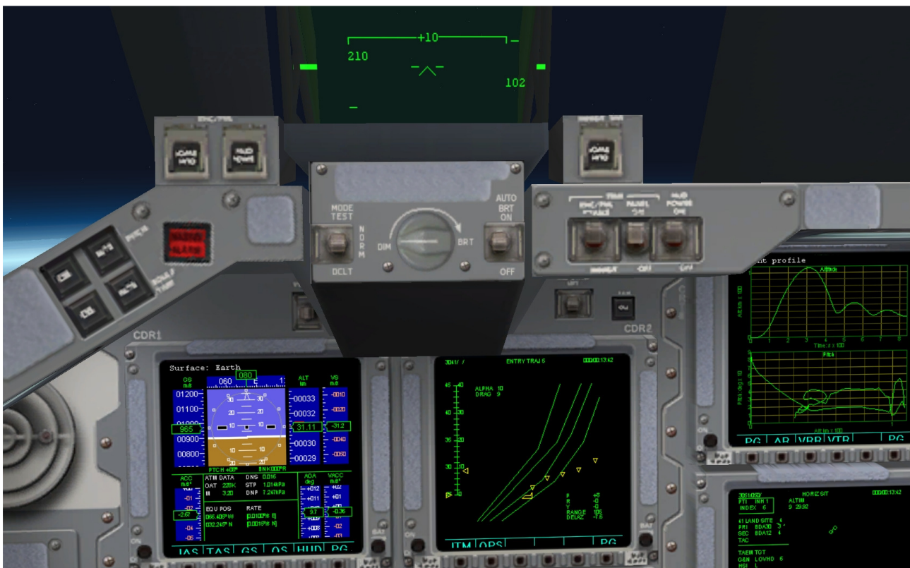
Fig.17 - TAEM. Note the phugoid profile performed by the Orbiter on the Ascent MFD
