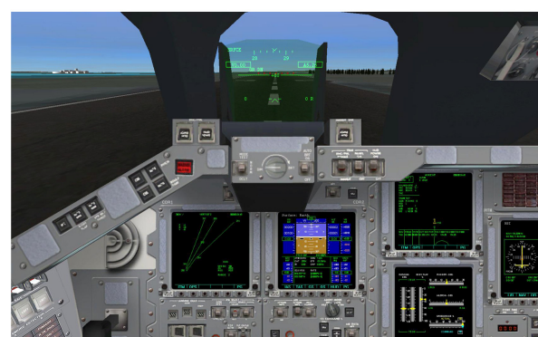
Fig.22 - Up/down and left /right the final to touchdown sequence - Note the HUD info displayed
