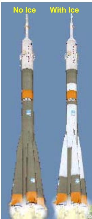
See at the beginning of this manual, the Soyuz launcher changes its color during the final launch sequence because the cooling of the tank forms ice on the external side.
