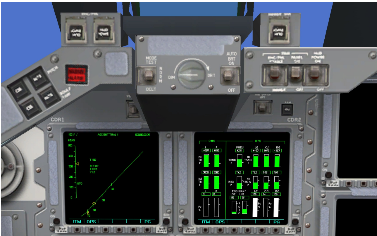
Fig.7 - Engine n.1 failed 30" after liftoff. Thrust on the good engines is automatically set at 109%. The Orbiter keeps flying the normal ascent profile while "Abort RTLS 2+30" is invoked by MCC. This means no action will be required until that time after SRB separation.
