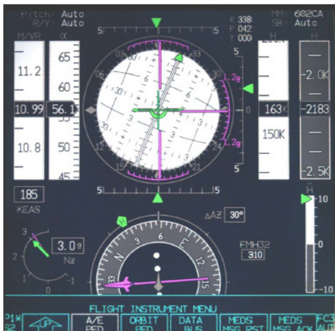
Fig.4 - The H' value (-2183 fps) shows how fast the orbiter is descending during NzHold phase.
