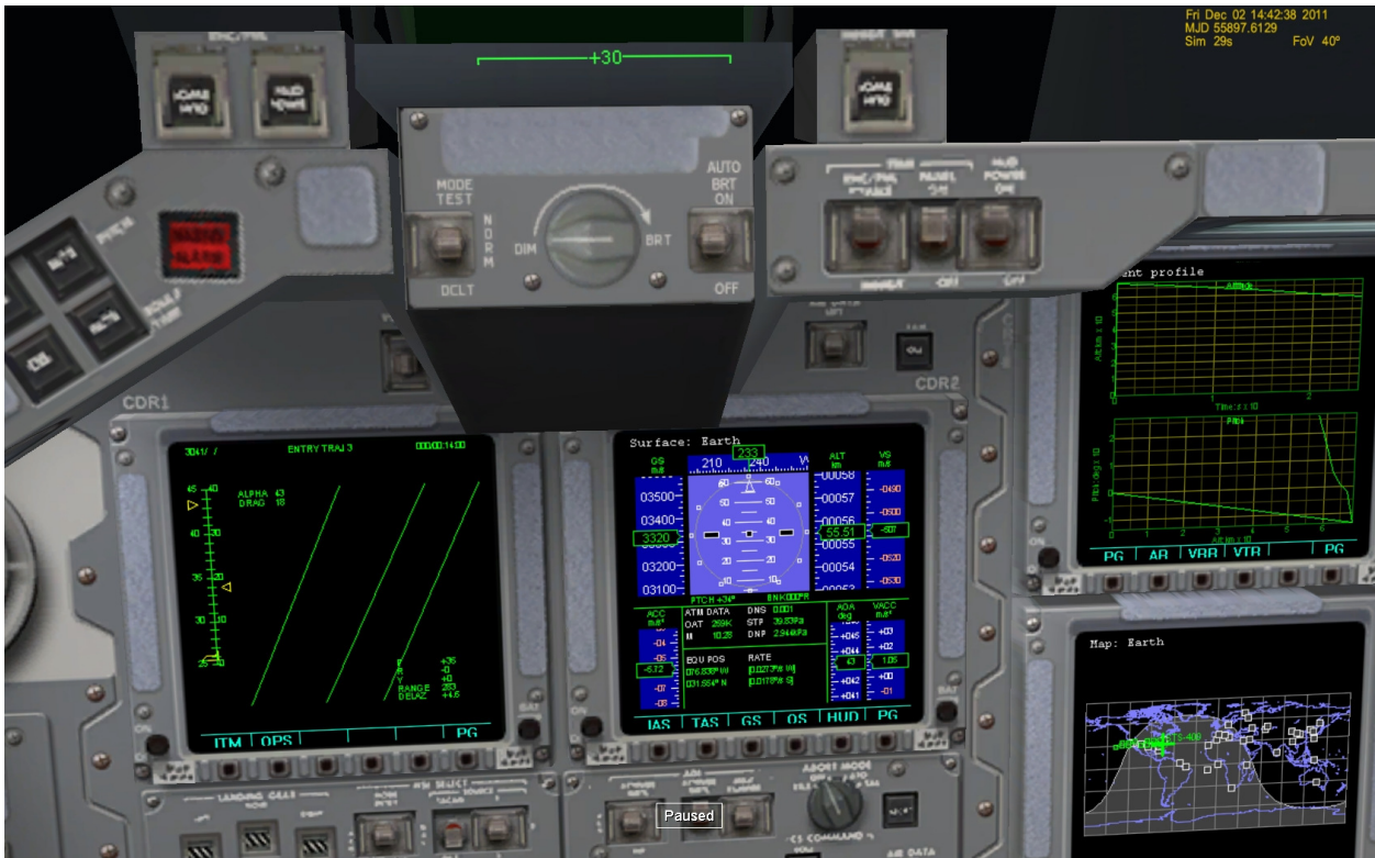
Fig.12 - Alpha recovery: note AoA around 50° and Acc increasing
