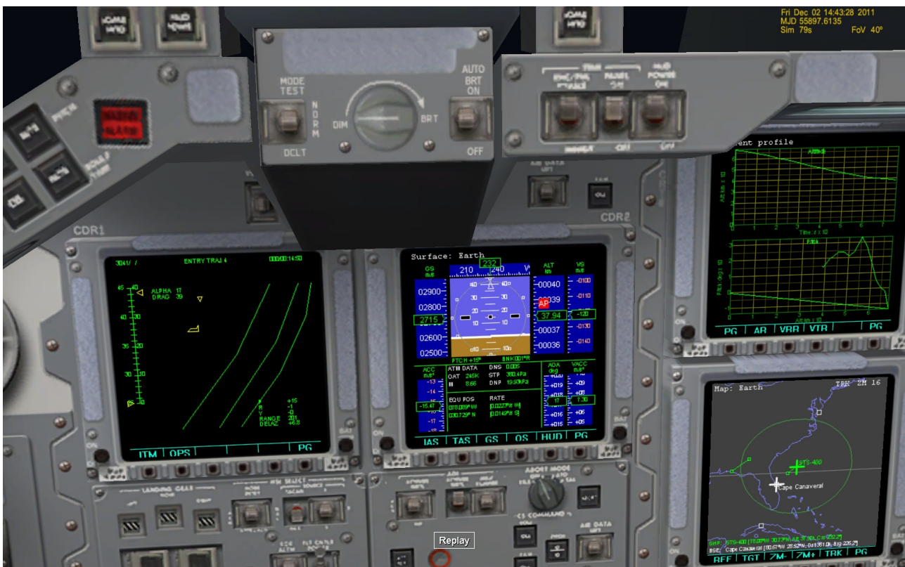
Fig.13 - Orbiter 200NM from KSC during Nz Hold phase: AoA is decreasing to keep 2.2g max.
