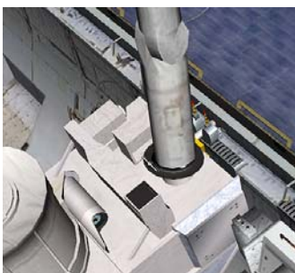
Correct position for the RMS for gripping CRISTA
