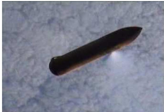
After ET SEP the orbiter will perform a roll maneuver so the upper windows point towards ET, in order to inspect it and take pictures to analyze damage during ascent.
