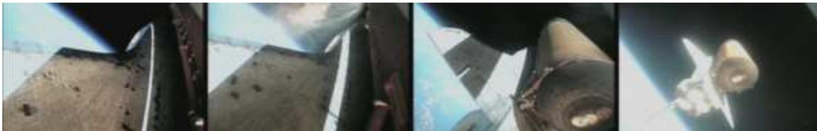
After about 8 minutes of flight, when apoapsis has been set and the craft has reached a certain velocity, it comes the time to turn of the SSMEs that use fuel from the External Tank (ET).
