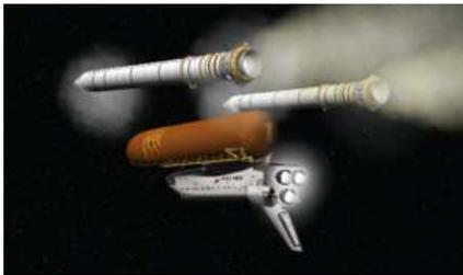
After 2 minutes of flight, the Solid Rocket Boosters (SRB) will detach from the craft at an approximate altitude of 43km above sea level. This point is designated as SRB SEP.
