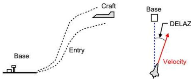
S-Turns will cause changes in the DELAZ (Delta Azumit) angle, and would make the craft to lose energy so it does not bounce back to space.
