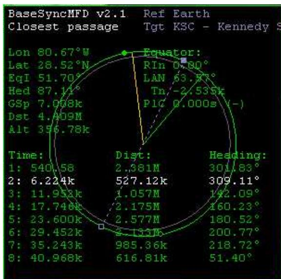
We need to pass over the landing site in the near future, which means that the closest pass in a certain orbit will be near zero. Closest pass is exactly what BaseSync calls "Dist". It has 3 columns but we only need 2:
