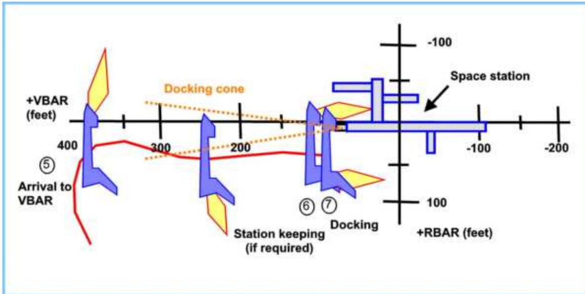
This maneuver is about placing ODS along the VBAR axis to dock with space station. Once you start this maneuver you may use Docking MFD, since you will be inside the docking cone and you have a signal coming from the docking port.
