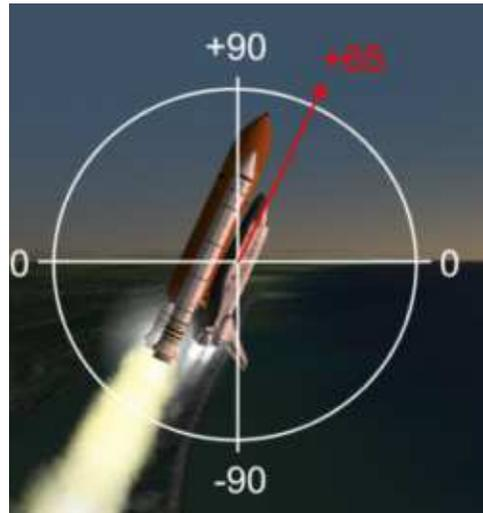
Use keypad 2 and 8 to control your pitch angle. Notice how GPC also has markers that indicate the pitch angle you should have at a certain moment. Maintaining the right pitch is very tricky.
