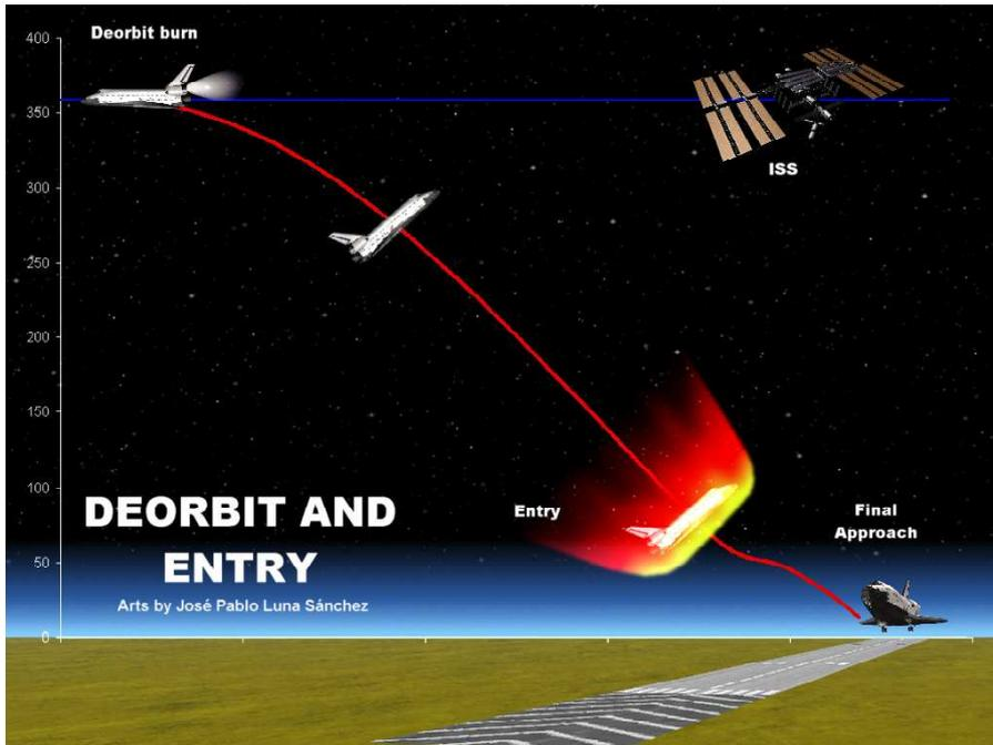
Deorbit is the process of lowering periapsis inside the atmosphere, using a retrograde burn, so we start the descent. Once you touch the atmosphere you start EI (Entry interfase) where you will perform an aerobrake maneuver to put the point of impact right on the landing site.
