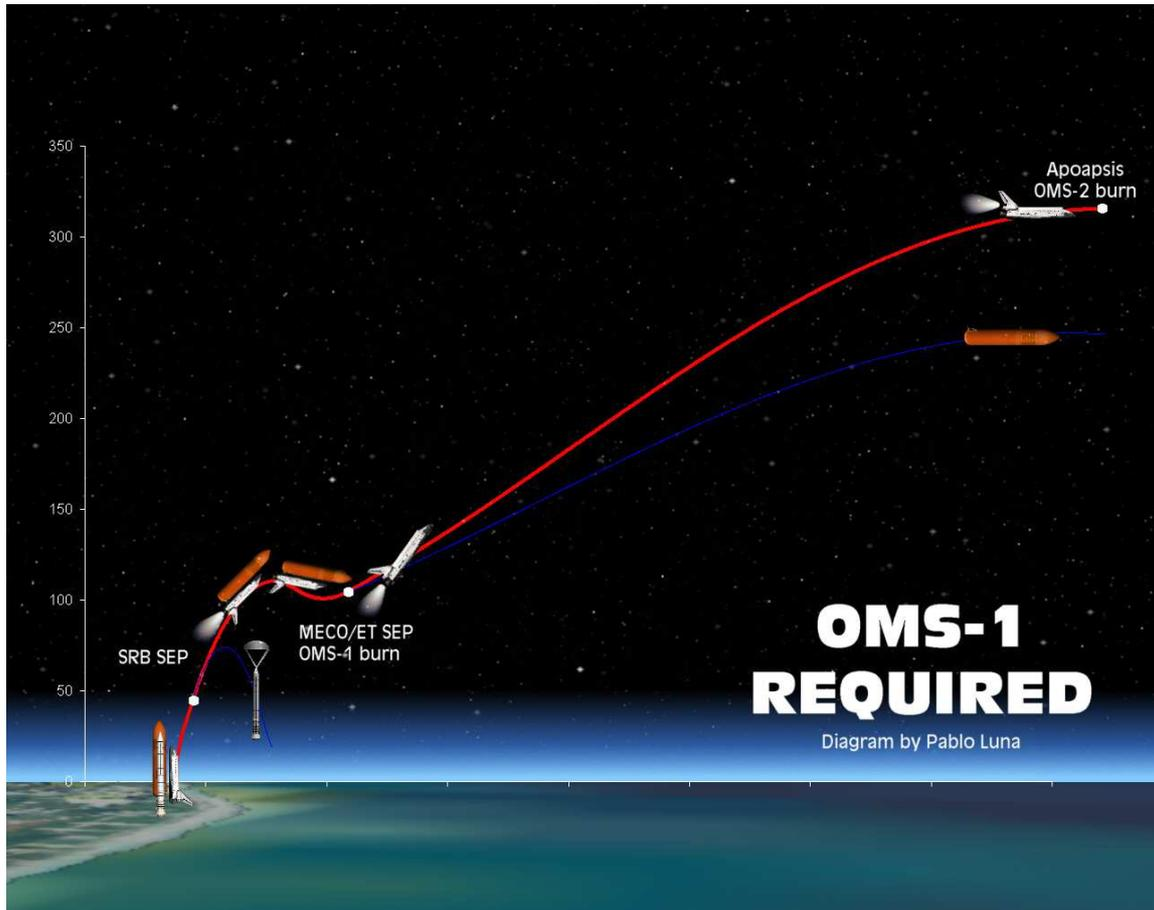
In this profile the craft remains inverted during MECO and ET SEP. After ET SEP, the orbiter will conduct an OMS-1 burn to raise apoapsis, and as it gets close to apoapsis a prograde OMS-2 burn takes place to circularize the orbit.
