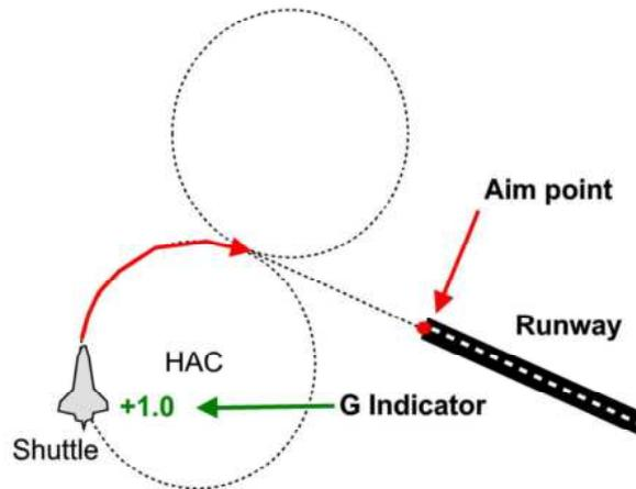
HAC stands for Heading Alignment Cylinder and it helps you to be perfectly aligned with runway as you intercept the cylinder and start turning around it.
